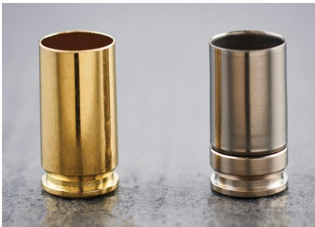
Pretty sure we don't need to tell you which is which. Note the seam between nickel alloy body and aluminum base. Photo by A1F Staff.
